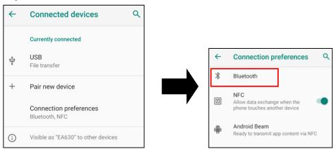
Tap **ON / OFF** to enable / disable Bluetooth®. To pair the available device, turn Bluetooth® ON to choose the available device.
