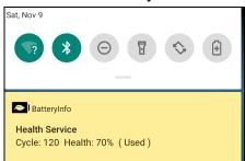
■ When the battery health is lower than 60% : (Battery should be replaced)
