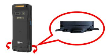
2. And pull the battery up to remove it.
