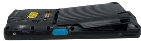
2. Press and hold both of the plastic buckles at the bottom, then push against the front.
