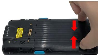
2. Push the battery against the front and lift to remove.
