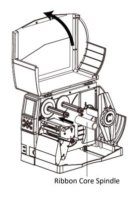
2.Load the outside ink ribbon into ribbon supply spindle, then anticlockwise tighten the latch knob to fix the ribbon.
