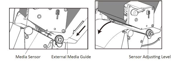
4. When using the gap label, black mark label or punch hole label, you can manually adjust the media sensor by the pulling to find the gap, black mark or punch hole for the start printing position.
