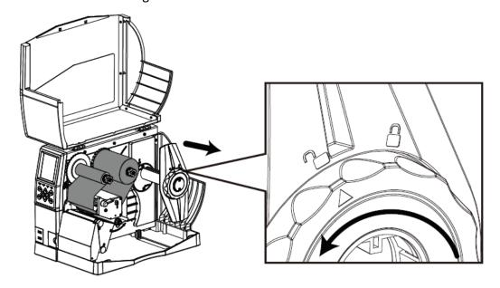
2. Mount a label roll onto the media spindle. Be sure to push the roll all the way aligned the inner wall of the printer. After the label roll be loaded, put the media guide back on the media spindle. Then rotate the arrow mark that locates in unlocking position to lock position so that it can be latched.
