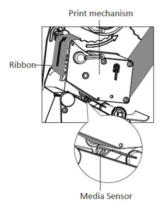
4. Pass the ribbon over the print mechanism and the ribbon take-up spindle, and then wrap it several turns around the ribbon take-up spindle.
