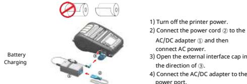
**!** The printer may incur serious damage if the AC/DC adapter provided by BIXOLON is not used. BIXOLON is not legally liable for any such damages.
