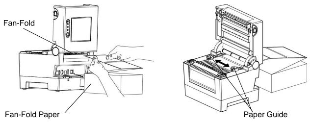
4) If you use Black-Mark or Notch paper roll, please lift up the paper and match the sensor position adjust the black mark or notch hole.
